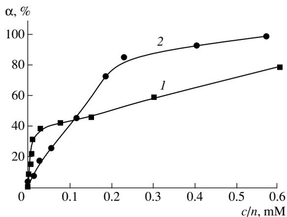
**Fig. 4.** Degrees of reduction of R-SG as functions of (1) Analgin and (2) ascorbic acid concentrations in solution.  $n = 1$  (ascorbic acid) or 20 (Analgin). pH: (1) 10.5 and (2) 9.3.  $m = 0.1$  g;  $V = 10$  mL;  $a = 5 \times 10^{-6}$  mol/g.
