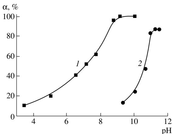
**Fig. 3.** Degrees of reduction of R-SG ( $3 \times 10^{-6}$  mol/g) with (1) a  $6 \times 10^{-3}$  M ascorbic acid solution and (2) a  $1.2 \times 10^{-2}$  M Analgin solution as functions of pH in solution.  $m = 0.1$  g;  $V = 10$  mL;  $a = 3 \times 10^{-6}$  mol/g.
