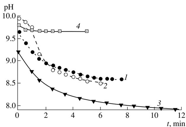
**Fig. 2.** Kinetic curves of pH changes on the addition of a sorbent in the systems: (1) silica gel–H<sub>2</sub>O, (2) silica gel–ascorbic acid solution, and R-SG–ascorbic acid solution (3) in the absence and (4) in the presence of a carbonate buffer solution. All solutions had pH 10.6 before the addition of the sorbent. The ascorbic acid concentration was  $6 \times 10^{-3}$  M;  $m = 0.1$  g;  $V = 10$  mL;  $T = 293$  K.
