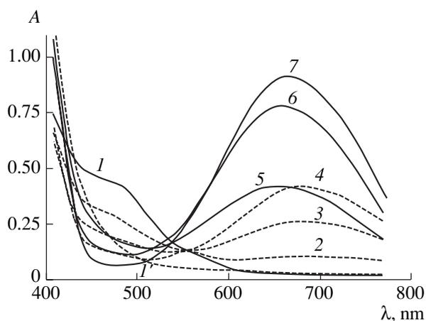
**Fig. 1.** Absorption spectra of a suspension of R-SG (1, 1') before and after treatment with (2–4) Analgin and (5–7) ascorbic acid solutions. Concentrations ( $n \times 10^4$ , M): (2) 1.6, (3) 12.6, (4) 120, (5) 1.14, (6) 2.27, and (7) 5.68. pH: (1–4) 10.5 and (1', 5–7) 9.3.  $m = 0.1$  g;  $V = 10$  mL.
